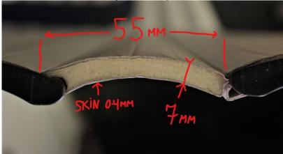
3. Roller shutter for openings spanning up to 1700mm width.
