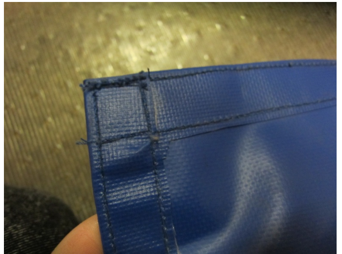
Examples of lapping the edges
