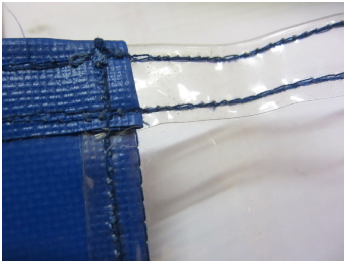
Examples of lapping the edges
