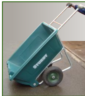
2. Lift handles of barrow until the bucket tilts forward away from the frame.
